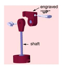
1. Join the components so the ball of the shaft is directed away from the flat surface of the grip marked "UP".
