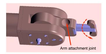
2. Insert the arm assembly into the attachment joint until the telescoping inner rod will allow for the required manipulator movement.
