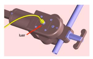
1. Connect the single gas line to the main pivot luer.
