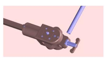
3. Tighten the main pivot handle clockwise.
