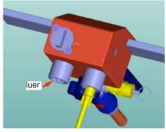
2. Connect the other end of the single gas line to one of the gas output luers of the supply module.
