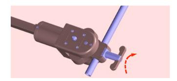
Stops prevent the arm from falling prior to pressurizing the system. Do NOT overcome these stops.
