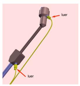
3. Connect the branched line to the two luers of the arm assembly.
