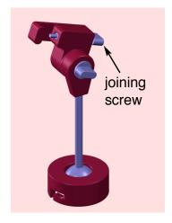
2. Position the manipulator joining screw so the adapter can be joined to the manipulator.
