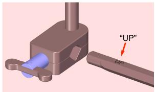
3. Insert the cross rod into the connection joint.
