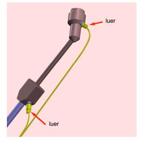
3. Connect the branched line to the two luers of the arm assembly.
