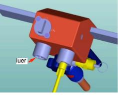
2. Connect the other end of the single gas line to one of the gas output luers of the supply module.
