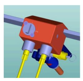
4. Connect the other end to the remaining luer of the supply module.
