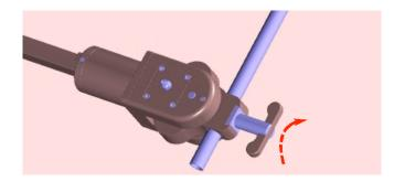
Stops prevent the arm from falling prior to pressurizing the system. Do NOT overcome these stops.
