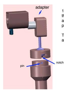
1. Connect the adapter to the arm by sliding the two adapter notches over the two arm pins and rotating the adapter clockwise. Gas pressure must be off during this step.
