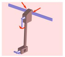
When placing the Sidekick Rail Grip onto the table rail, do not put it over the rail table attachment or a table rail notch.
