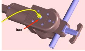
1. Connect the single gas line to the main pivot luer.
