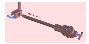
4. Slide the main pivot until the arm connection is located below the planned connection to the manipulator.
