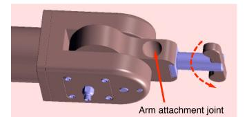
2. Insert the arm assembly into the attachment joint until the telescoping rod will allow for the required manipulator movement.
